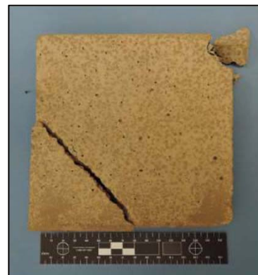
Martian simulant JSC Mars-1A, MgO-MKP cement, boric acid (set retardant*) and water – sample fractured during shipping to JSC prior to testing
