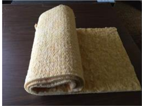
Figure 10. UPF Insulation. This lightweight fiberglass batting is the Gen 2 baseline insulation.
