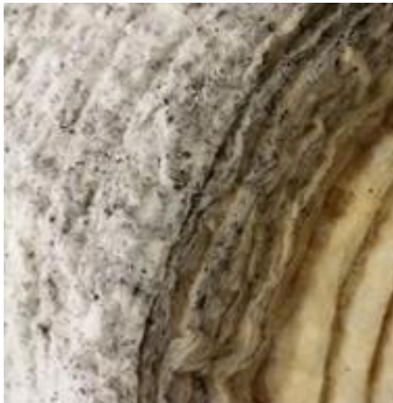
Figure 11. UPF Insulation with Embedded Intumescent Graphite Flakes.
