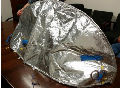
Figure 6. Thermal Pod Design. Alternate CHIEFS shelter design with more efficient use of surface area.
