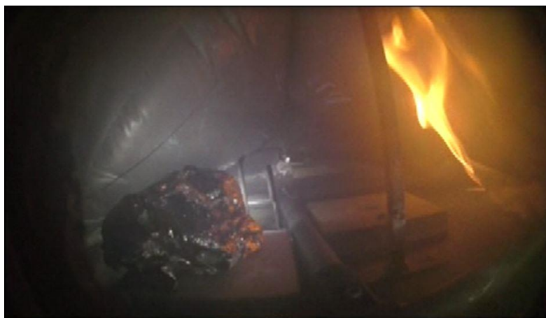
Figure 7. Open flames within CHIEFS shelter. Flames in this shelter are entering underneath the shelter floor band, this was a common point of flame ingress.
