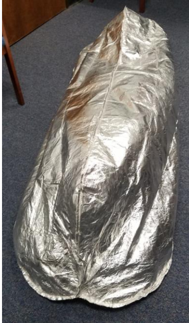
Figure 13. MW shelter. The MW geometry is similar to the M2002 but uses less total running seam length.
