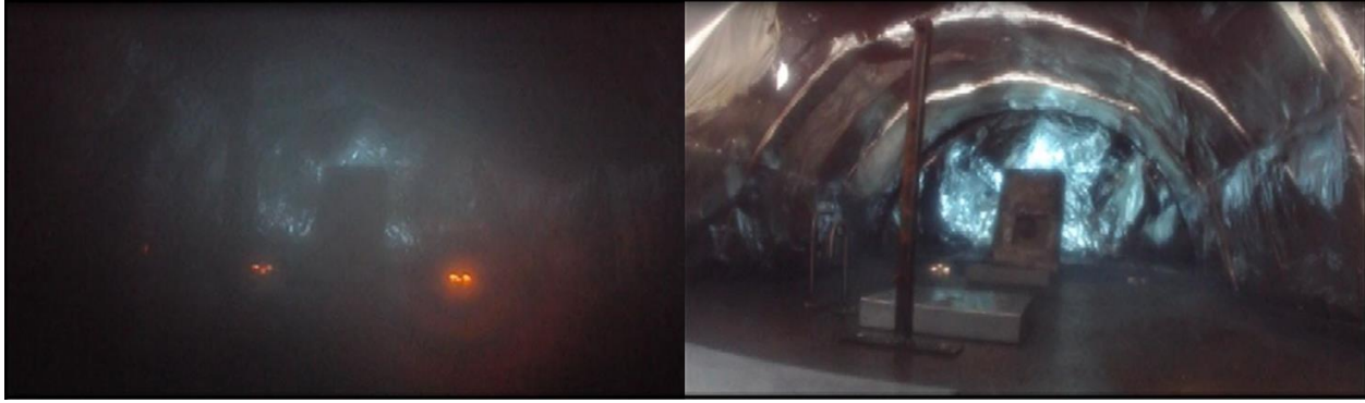
Figure 8. M2002 shelter self ventilating. Approximately 20 seconds into the test the M2002 visibly accumulates flammable thermal decomposition byproducts (left); at the conclusion of heating – approximately 60 seconds into the test – the M2002 gas barrier is severely compromised and thermal decomposition byproducts easily ventilate outside of the shelter (right). This is likely the reason explosive flashes were not observed within the M2002.
