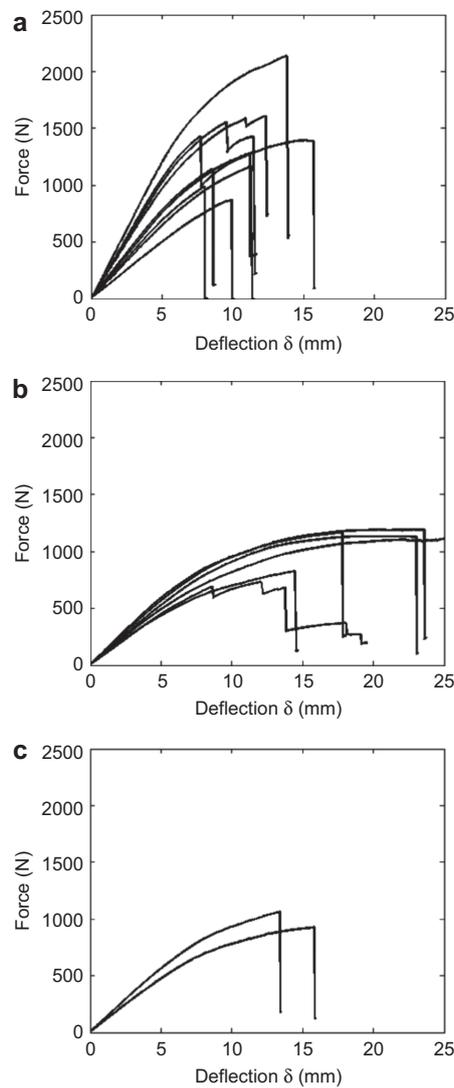
**Figure 3** Force-deflection curves from small samples loaded in FPBT: (a) yew YEW<sub>b</sub>, (b) juniper JUN<sub>b</sub>, and (c) pine PINE<sub>b</sub>.
