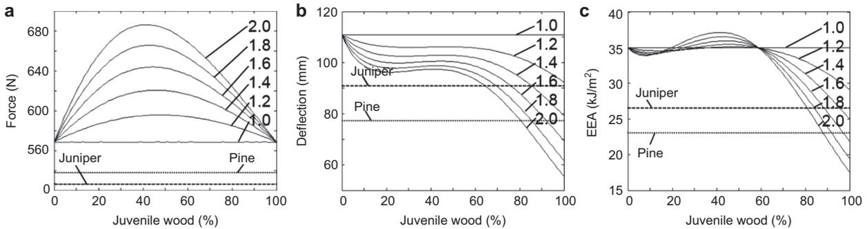
**Figure 4** Theoretical values as a function of juvenile wood moiety in a longbow model: (a) force, (b) deflection, and (c) EEA. The cross-section is set to consist of juvenile wood on the compression side (“belly”) and mature wood on the tension side (“back”). See Figure 1a–c. The stiffness of the juvenile wood is a factor  $n$  stiffer compared with the mature wood, where  $n$  is varied from 1.0 to 2.0.
