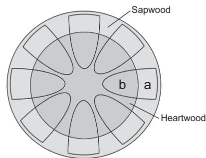
**Figure 5** Optimized utilization of the material, which not necessarily results in optimized performance of the bow: positioning of the D-shaped bow cross-sections in the yew stem: (a) back side (tension) and (b) belly side (compression).
