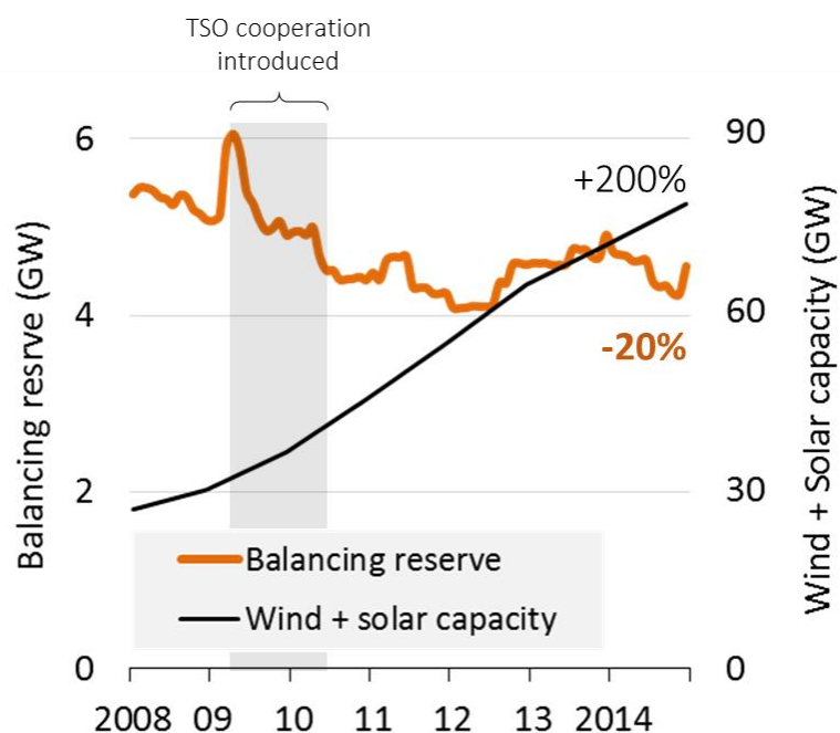
Figure 7. Balancing reserves (SC + TC, average of positive and negative reserve) and VRE capacity (wind + solar) in Germany. Even though the installed capacity of wind and solar power has tripled since 2008, the demand for balancing power has decreased. One reason was the cooperation between TSOs introduced in 2009/10.
