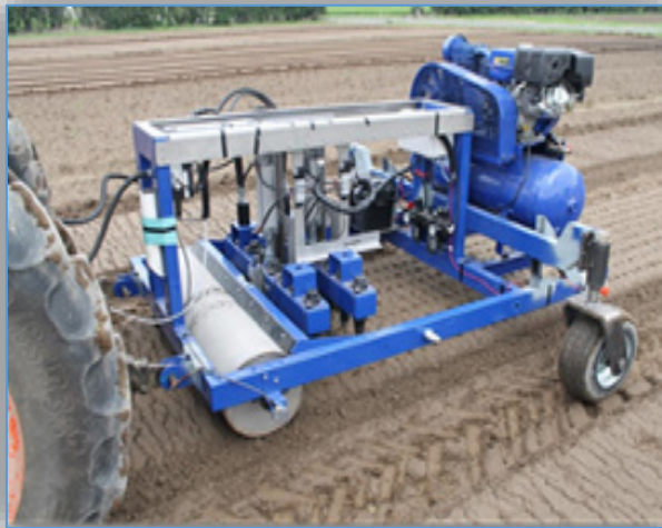
Figure 5 – Completed mechatronic dibbling machine during testing
