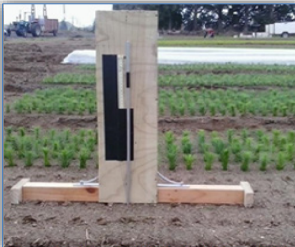
Figure 6 – Measuring device for hole depth and angle
