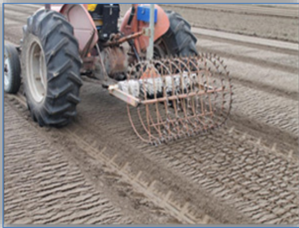
Figure 2. Radiata Pine dibbling machine
