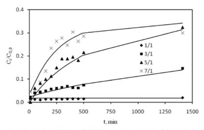
Figure 3. Experimental and estimated C<sub>i</sub>/C<sub>0.0</sub> of 1,3-DNG at various mole ratio of nitric acid/glycerol (nitric acid of 69%, temperature of 20 °C)
