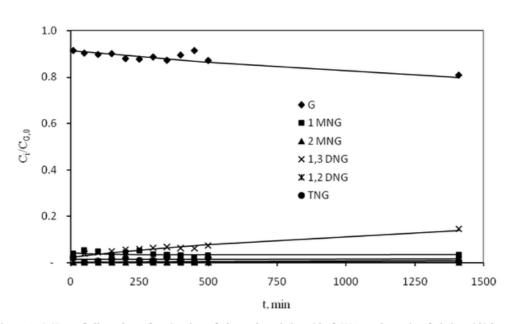
Figure 1.  $C_i/C_{G,0}$  of all products for nitration of glycerol at nitric acid of 69%, molar ratio of nitric acid/glycerol 3/1 and temperature of reaction 20 °C
