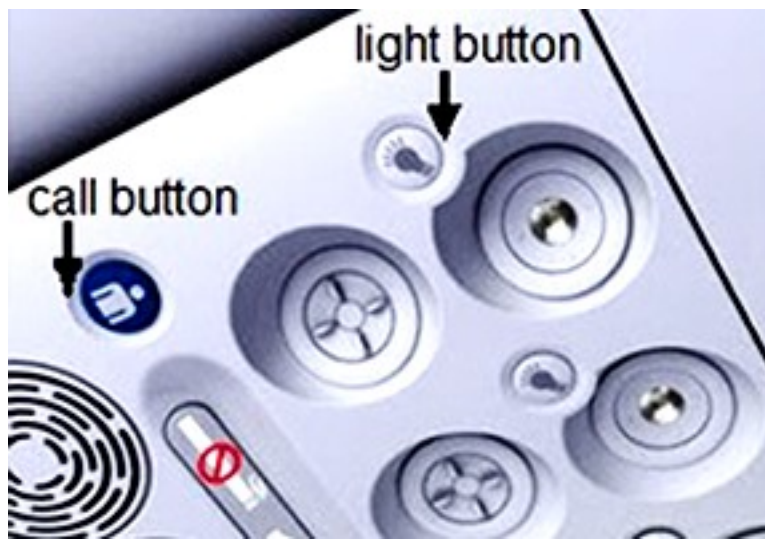
Figure 4.4. Boeing 737 flight attendant call button Source: Primm, 2011
