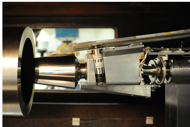
Figure 2. Cone model installed in SLDT. Diffuser capture not installed for this image.
