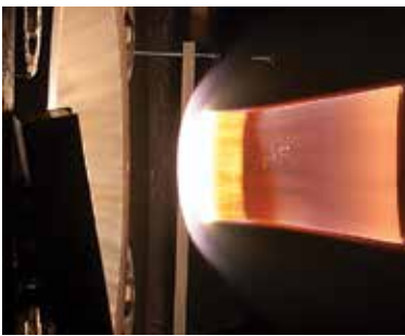
Testing of HEEET material at the NASA Ames Arc Jet Complex in the Interaction Heating Facility.
