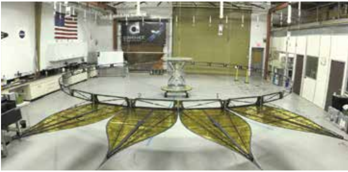
A 10-m prototype of the starshade's inner disk is demonstrated at NASA's Jet Propulsion Laboratory.
