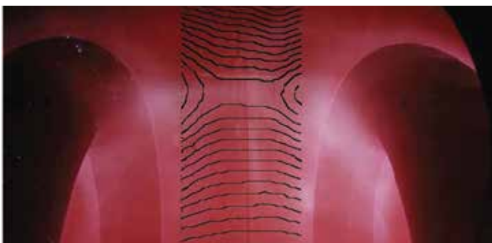
Photo of a hydrogen plasma where magnetic reconnection is generated in MRX by two coils (blackened objects on the left and right), superimposed by reconnecting magnetic field lines measured by in situ diagnostics.
