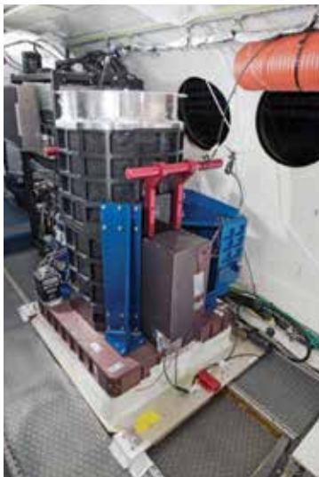
The 2 micron IPDA lidar system installed in the NASA B200. (Image credit: Upendra Singh)
