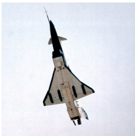
The X-31 at high AOA in Paris; note the position of the canards. (Rockwell)
