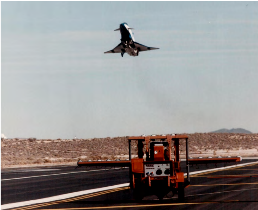
X-31 flying a simulated carrier approach at Edwards AFB using a Fresnel Lens Optical Landing System reference system. (NASA DFRC)
