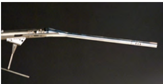
Kiel probe canted to compensate for high angles of attack. (NASA DFRC)
