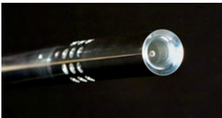
Kiel probe “collar” to “collect” pitot pressure at high AOA. (NASA DFRC)
