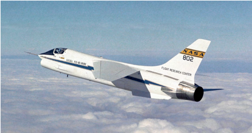
F-8 digital fly-by-wire test bed, 1972. (NASA DFRC)
