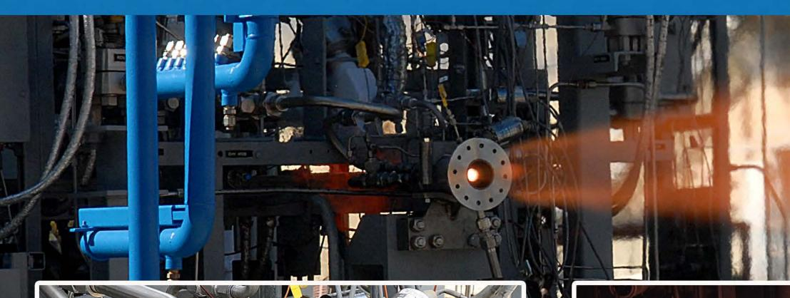
Hot-fire testing has demonstrated parts manufactured with this technique can survive and perform well in the relevant environments for liquid rocket propulsion systems.
