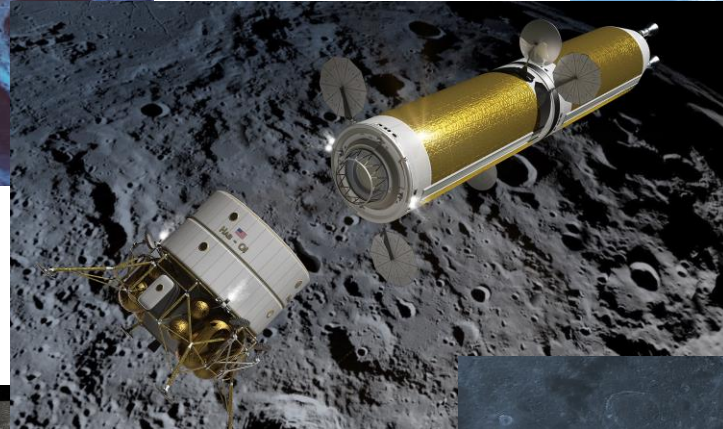
Reusable Lunar Cargo Transport uses 3 – 16.7 klb f "SNRE-class" Engines – (2013)
