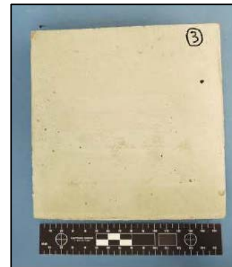
Lunar simulant JSC-1A, stucco mix, OPC, and water
