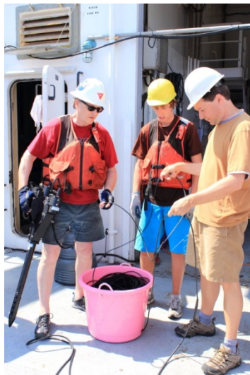
Figure 1: The author (left) preparing to launch the Satlantic Hyperpro aboard the R/V Kilo Moana.
