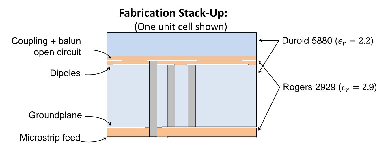
The impact of the groundplane and integrated balun is shown, demonstrating how the balun serves to increase bandwidth as an additional matching stage:
