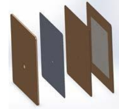
3D Printed RFID Antenna, layers
