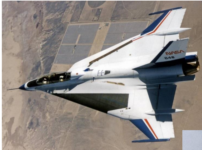
AFTI/F-16XL2 Supersonic Laminar Flow Control Glove and Attachments
