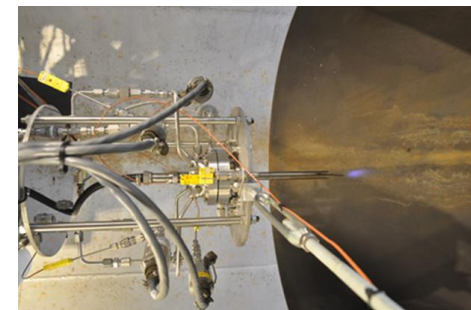
ASI Igniter testing at GRC ACS
