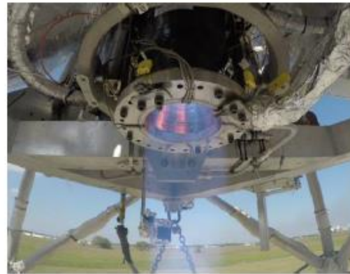
Cold He heat-exchanger on Morpheus
