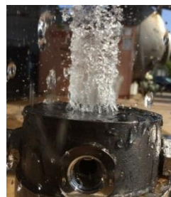
GG-Injector Water Flow Testing
