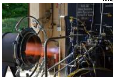
Aerojet Rocketdyne RL-10 engine thrust chamber assembly and injector
