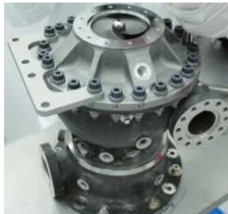
MSFC rocket engine fuel turbopump
