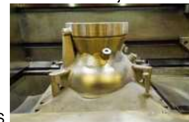
Commercial Crew Program SpaceX SuperDraco combustion chamber for Dragon V2
