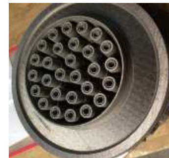
MSFC 28-element Inconel 625 fuel injector
