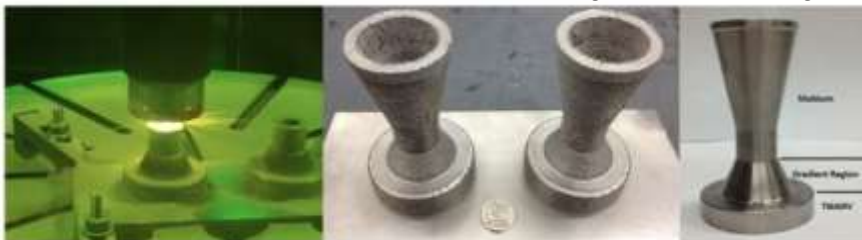
JPL Prototype titanium to niobium gradient rocket nozzle
