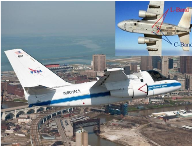
Figure 2 – Lockheed Orion S-3B research aircraft. Inset: antenna locations
