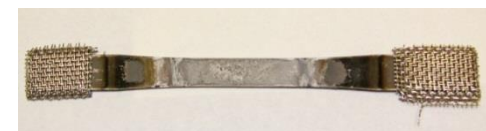
PVD GdYbYSi coated on Prepreg SiC/SiC 1316°C, 15ksi, 1169 h fatigue (3 Hz, R=0.05)
