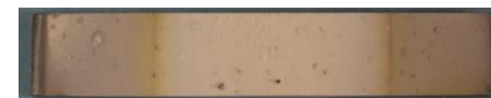
NASA 2700°F(1482°C)+ EBC System 188 on SA Tyrannohex SiC Composite, 1482°C 15 ksi, 500hr
