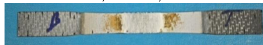
EB-PVD (Hf, Yb, Gd, Yb)_2Si_{2-x}O_{7-x} EBC/GdYbSi bond coat on CVI-MI SiC/SiC (with CMAS) 1537°C, 10ksi, 300 h fatigue (3 Hz, R=0.05)
