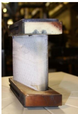
EBC Coated CVI SiC/SiC vane after 31 hour testing at 2500°F+ coating temperature
