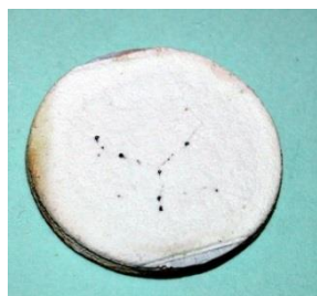
Interface Si bond coat melting of selected coating systems, under laser heat flux tests, 1" dia button specimen
