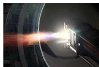
Sulzer Triplex Pro system having high efficiency and high velocity processing
