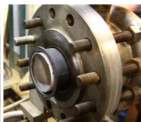
EBC Coated Rig Inner and outer liner testing 2500°F, 10-16 atm, completed 250 h
