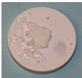
EB-PVD Low k \text{ZrO}_2\text{-}4\text{mol}\%\text{Y}_2\text{O}_3\text{-}3\text{mol}\%\text{Gd}_2\text{O}_3\text{-}3\text{mol}\%\text{Yb}_2\text{O}_3 /PtAl/Rene N5 (Howmet Processing- Run 3844, ID 15H1)
