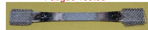
PVD GdYSi coated on Hyper Them CVI-MI SiC/SiC 1316°C, 10ksi, 1000 h fatigue (3 Hz, R=0.05)
