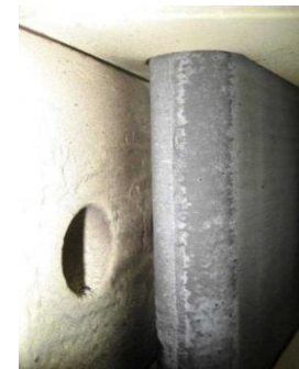
Uncoated vane tested 15 hr
