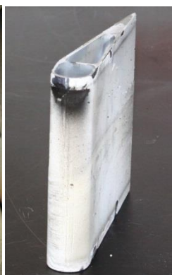
EBC Coated Prepreg SiC/SiC vane after 21 hour testing at 2500°F
