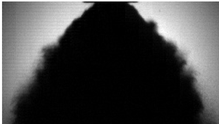
Figure 4. Example shadowgram of flow field created from the pressure swirl atomizer of liquid nitrogen flow collected at 40 kHz with a spatial scale of approximately 30 mm by 50 mm.
