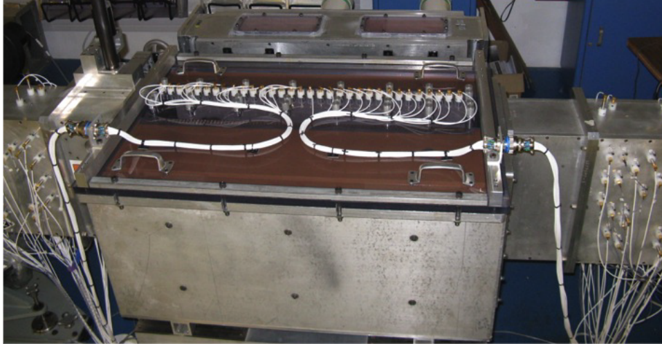
Figure 4: Photograph of Curved Duct Test Rig (CDTR) test section.
