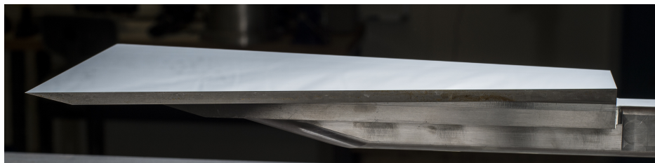
Figure 2. A side view of the polished flat plate. Measurement surface is toward the top of the picture.
