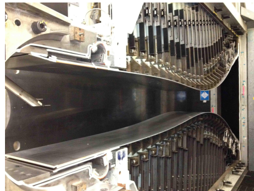
(b) Photograph of the NASA Langley 20 Inch Low Speed Wind Tunnel with the variable Mach number nozzle set at M=2 (Near side walls removed)
