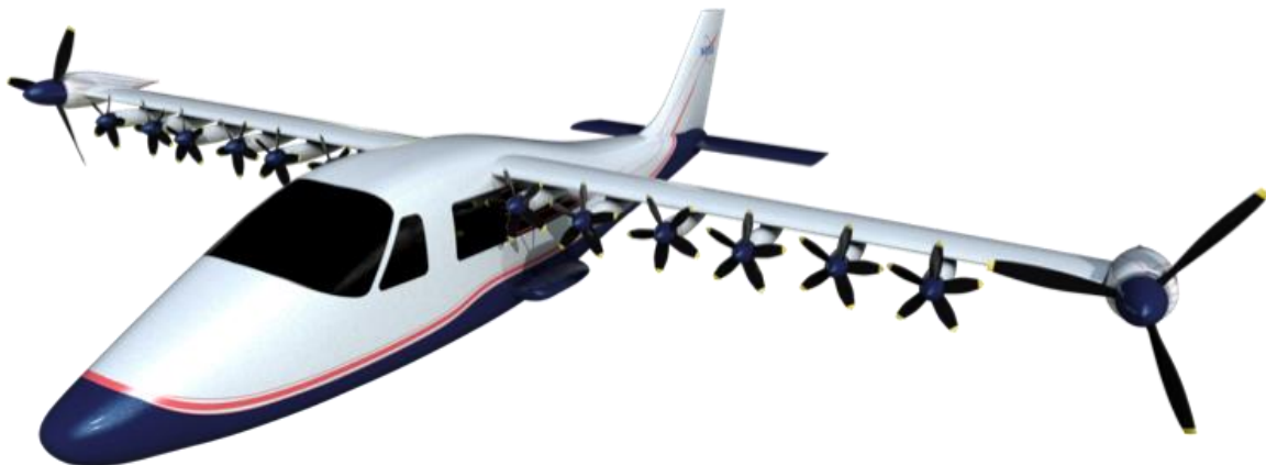
Figure 2. The X-57 Maxwell DEP aircraft. The Tecnam P2006T fuselage and tail with the DEP wing system that includes the wingtip propulsors and the DEP high-lift motors.
