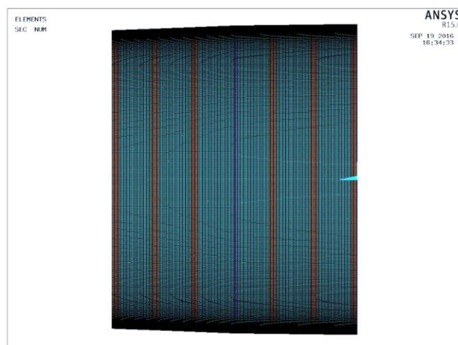
Figure 9: Finite element model; blue=beryllium aluminum, yellow=PMN bonded to beryllium aluminum, purple=simplified mount (zero displacement)
