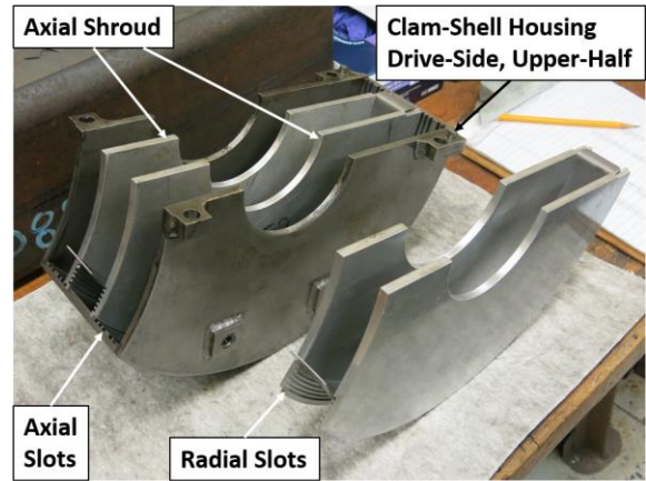
Figure 4 Configuration of axial and radial shrouding using machined slots.
