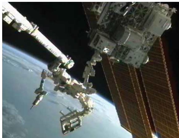
Fig 17: The Robotic Refueling Mission investigation (center, on platform) uses Canadarm2, the International Space Station's robot arm, and the Canadian Dextre robot (right) to demonstrate satellite-servicing tasks. (Image credit: NASA)
