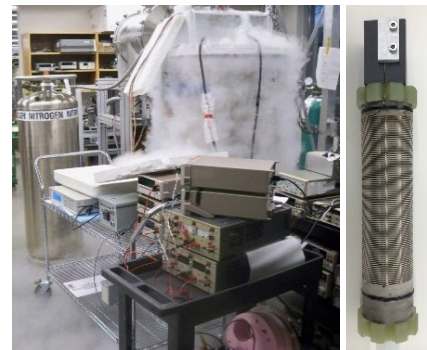
(b) CAPS idealized magnetic field test capability for wire segments
