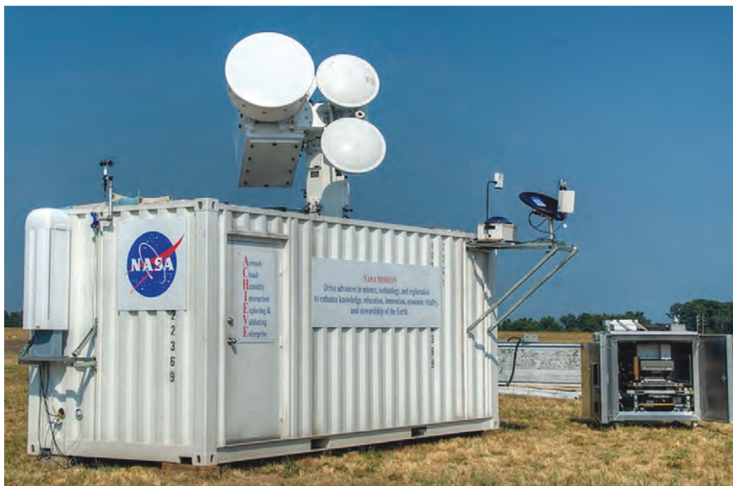
Figure 2.21: NASA GSFC's ACHIEVE radar.
