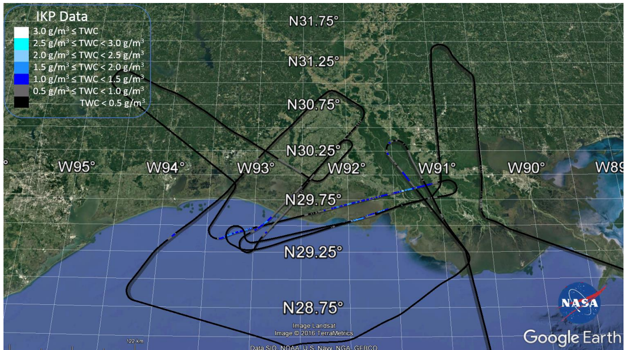
Figure 7. Flight path of DC-8 and measured ice water concentration from Ice Kinetic Probe for 19 August 2015.
