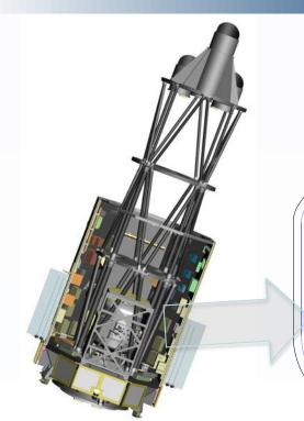
Soft X-ray Spectrometer used a microcalorimeter array operating at 50 mK
