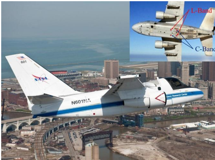
Lockheed Orion S-3B research aircraft. Inset: antenna locations
