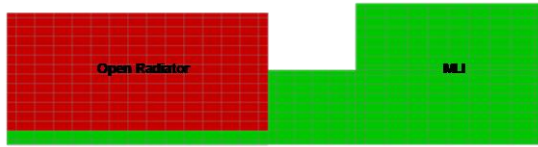
Figure 6. Cryo-Cooler Radiator Blanketing. Uncertainty in cryo-cooler performance results in large portion of cc radiator blanketed off. Radiator maintains capability to accommodate increases in cryo-cooler power
