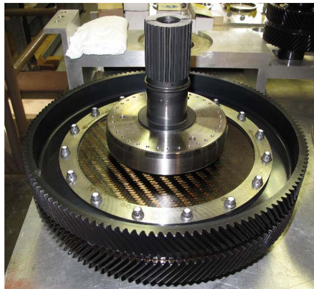
16.5 inch pitch diameter hybrid bull gear
