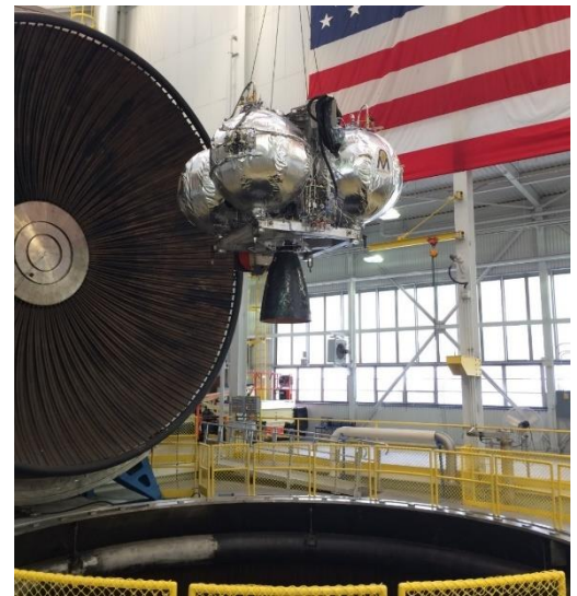
Figure 2: ICPTA test article suspended over the ISP test cell at NASA Glenn Research Center Plum Brook Station.
