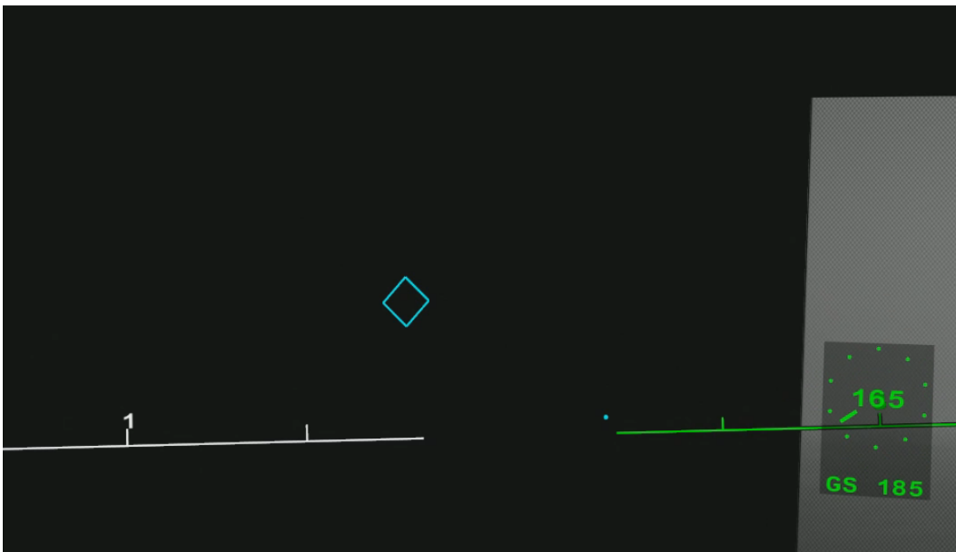
Figure 40. This figure is a screen capture of the pilot looking to the left of the Virtual HUD in IMC (notice the airspeed indicator of the Virtual-HUD on the right-side of the figure). The blue diamond symbology shows ADS-B traffic not in the forward field-of-view. The off-boresight 360° zero-pitch line is shown in white.
