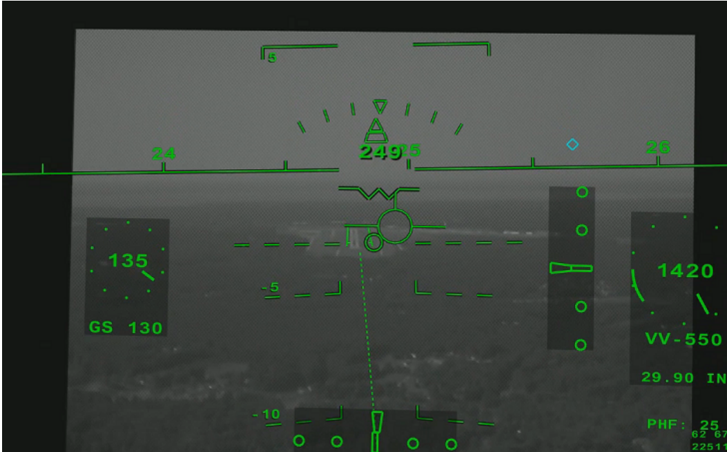
Figure 38. The flight symbology set overlaid on a simulated FLIR image. The blue diamond symbology depicted ADS-B traffic.
