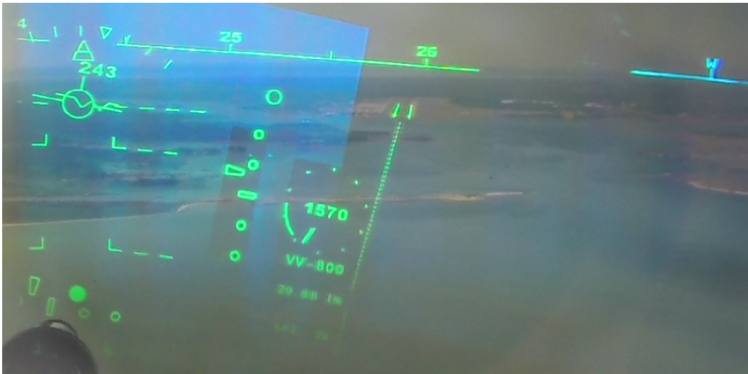
Figure 39. This figure is a screen capture of the pilot looking to the right of the Virtual HUD in VMC. The runway outline and extended centerline (dashed line) are shown in the middle of the figure to the right of the altitude dial. A partial view of the off-boresight 360° zero-pitch line is shown in white in upper right.
