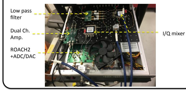
• Flux ramp frequency: 160 kHz, mixed frequency ~ 330 kHz
