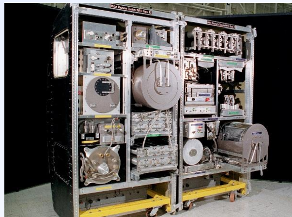
ISS Water Recovery System
