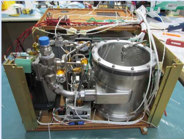
Pumped Separator for PBRE
