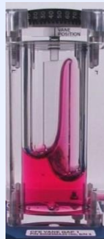
45° vane angle in microgravity.
