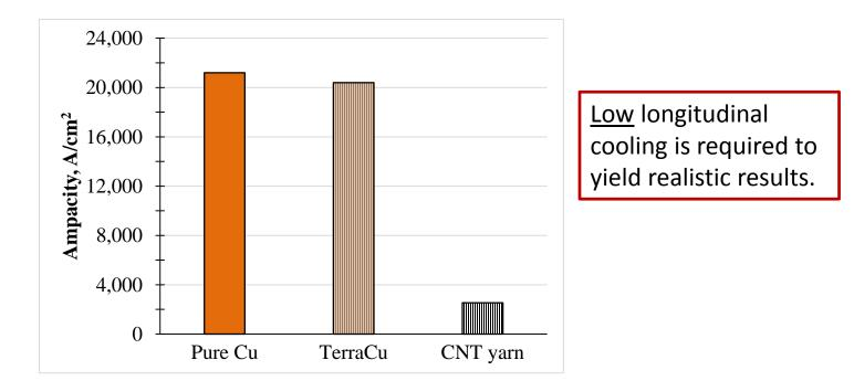
Average of 2 or 3 Ampacity measurements of Pure Cu, Cu-CNT composite TerraCopper, and a CNT yarn.
