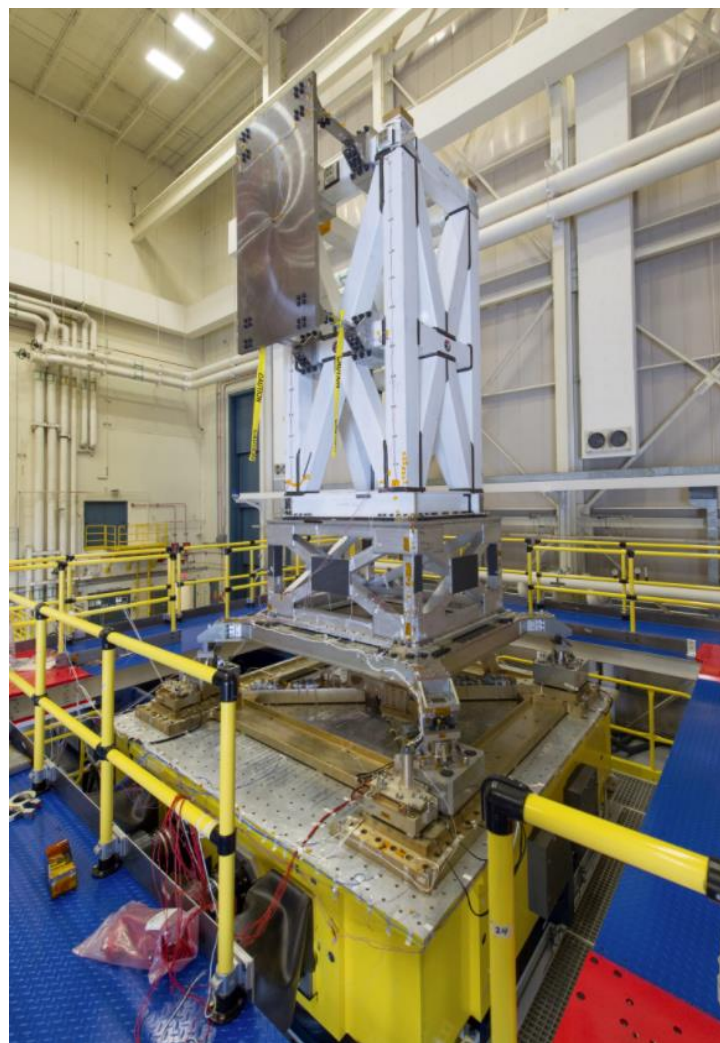
Vibration fixture with mass simulator on head expander for proof testing
