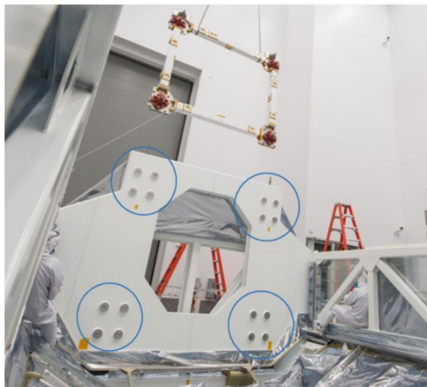
STTARS HIF interface locations (16 bolt holes)
