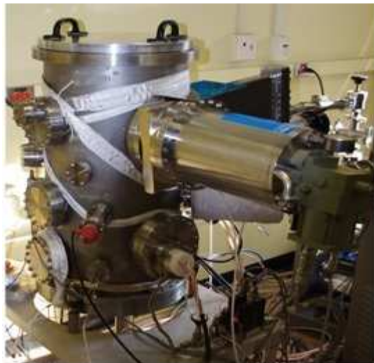
Figure 1. Image of the 0.5-meter vacuum chamber to be used for the Al deposition and fluorination experiments.
