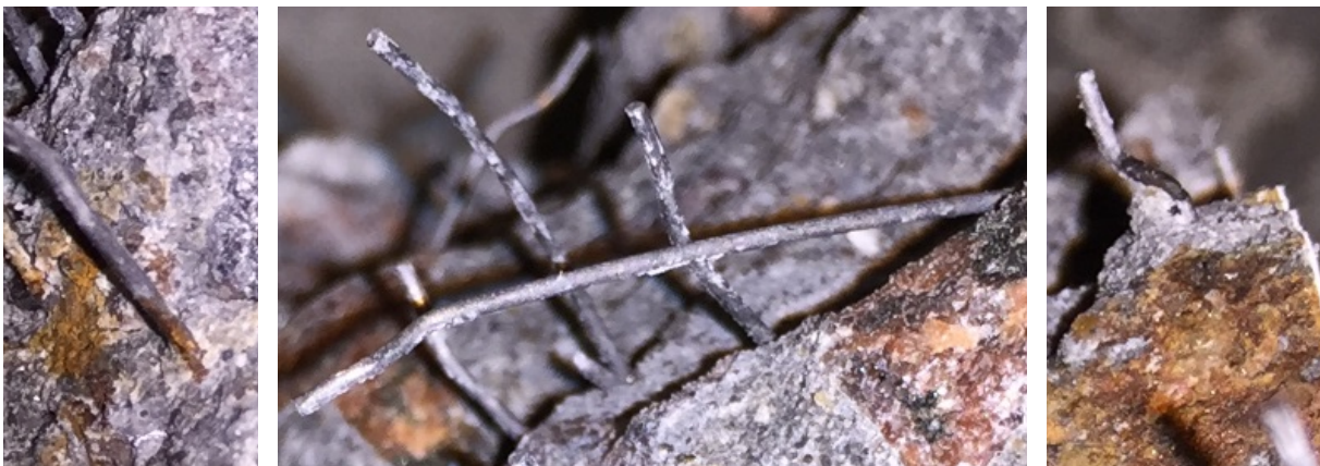
Figure 4.3. Example of the aspect of several embedded steel fibres in a loaded beam with a target crack width of 0.2 mm after three years of cyclic exposure to chloride solution.
