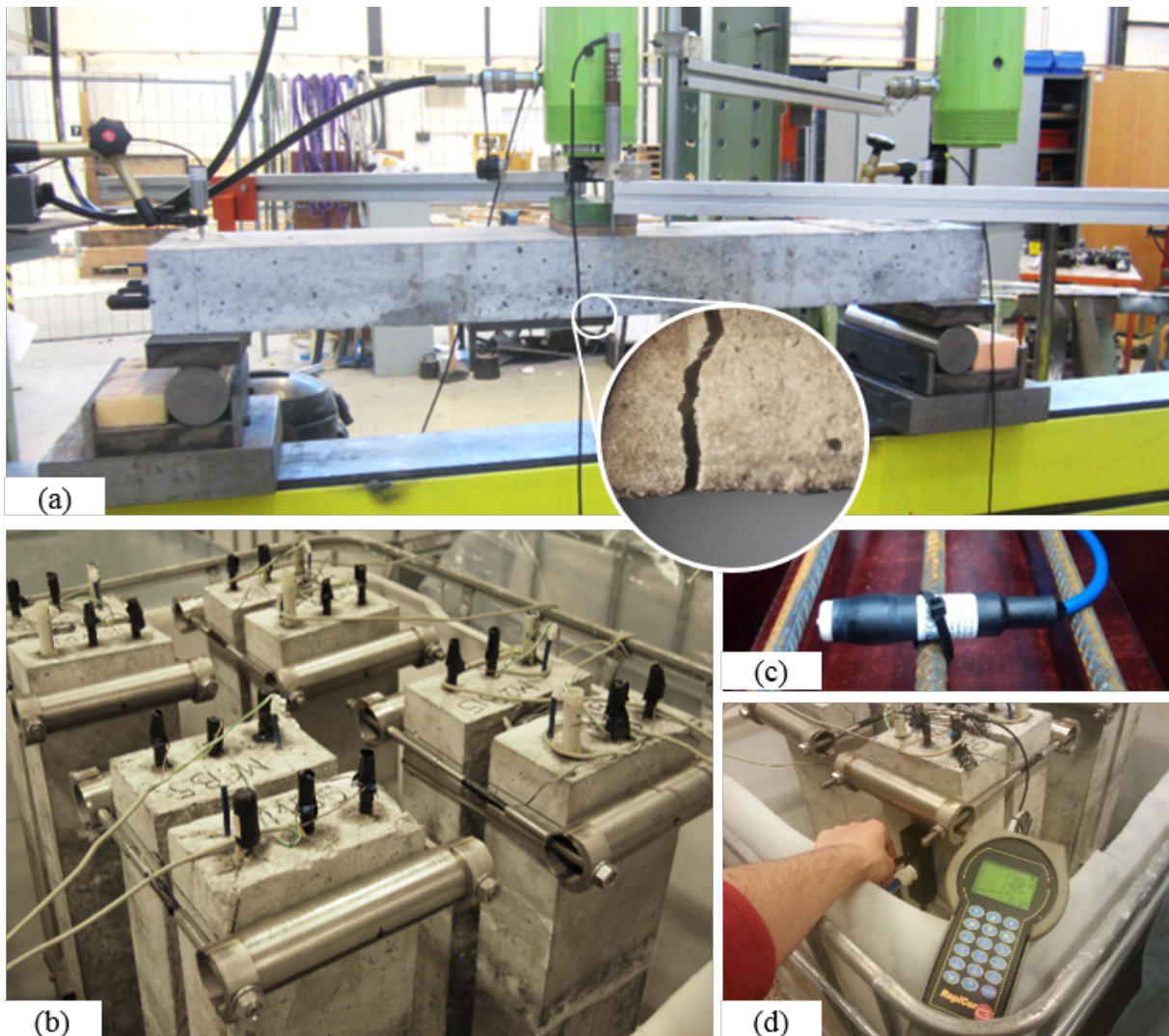
Figure 3.3. (a) Three-point bending procedure for pre-cracking of beams; (b) beams subjected to sustained load during exposure to chloride through partial immersion in a chloride solution; (c) embedded electrode ERE20 from Force Technology used for half-cell potential monitoring; and (d) monitoring of corrosion rates using the RapiCor device.
