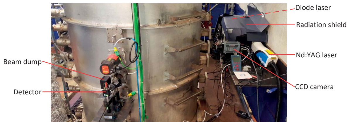
Figure 4. Experimental set-up during the latest campaign (described in Paper II) showing the different components used to perform measurements of the soot volume fraction in the Chalmers 100 kW oxy-fuel test rig. Note that the diode laser is beneath the radiation shield and the laser beams are directed through the flame onto the detector.
