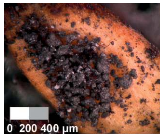
Figure 16. Particles collected from a co-firing flame. The white biomass particle is clearly much larger than the black coal particles.
