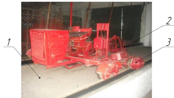
Fig. 2. General view of the sand test bed: 1 - soil, 2 - the coupling device of the discs, 3 - traction transfer device
