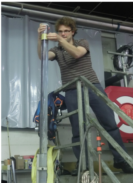
Figure 4 - a) Sampling form the SC using Beaker sampler; b) Piston.
