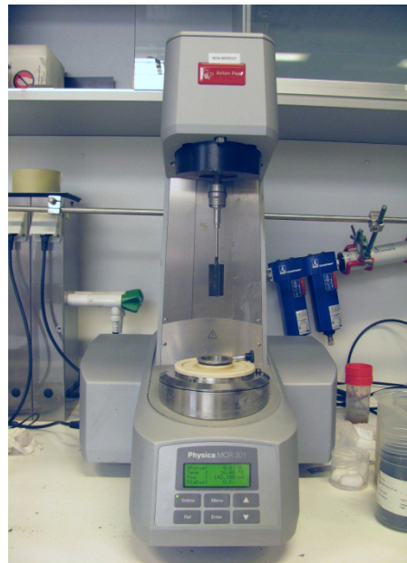
Figure 5 - The Anton Paar MCR 301 Rheometer of the Flanders Hydraulic Laboratory with the vane used in this research.
