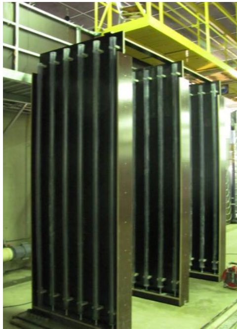
Figure 2 - Set of small consolidation columns for different harbors (SCs).
