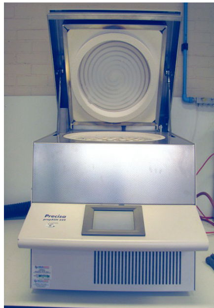
Figure 13 - Prepash device from the laboratory of FHR to derive dry matter, organic matter and carbonate content.
