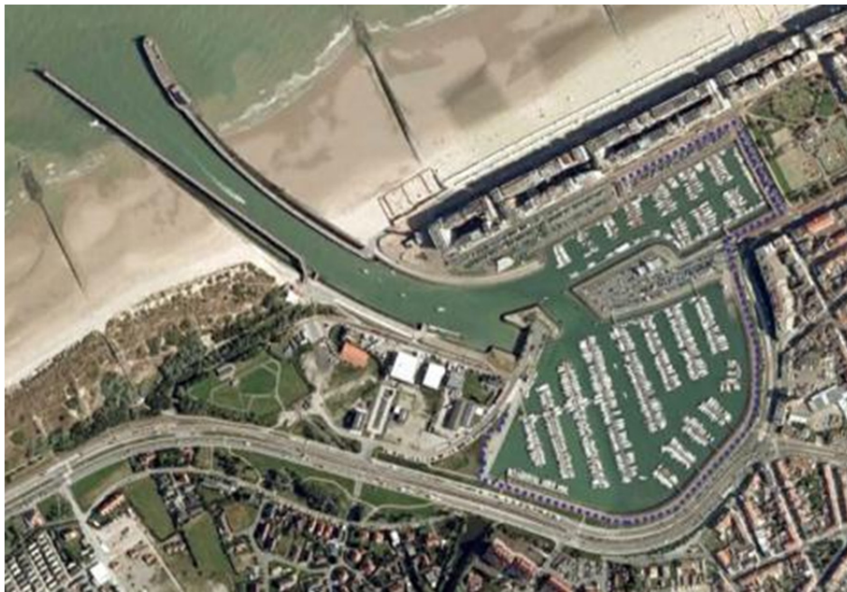
Figure 1-1: Trajectory of the water and wave retaining walls in the harbour of Blankenberge (Coastal Division, 2011). Along the western part of the northern quay, there already exist some walls.
