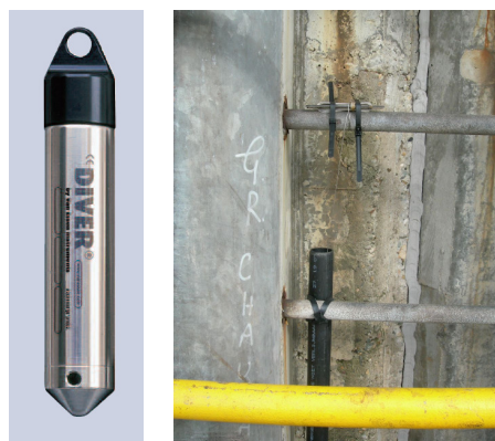
Figure 7 : Water level sensor (left) mounted in ladder recess of lock chamber wall (right)
