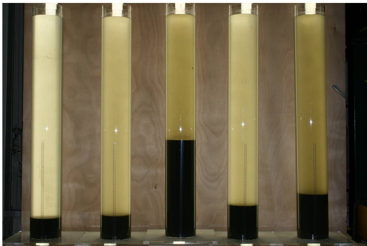
Figure 3.14: Example of image captured with CANON digital SLR (3888 x 2592) to determine interface settlement. Column height = 1 m; ruler length = 0.20 m; distance between two ruler ticks = 0.01 m.
